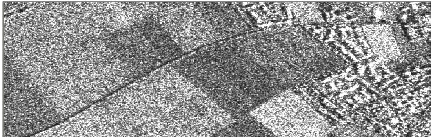
Appearance of speckle noise in TerraSAR-X data
